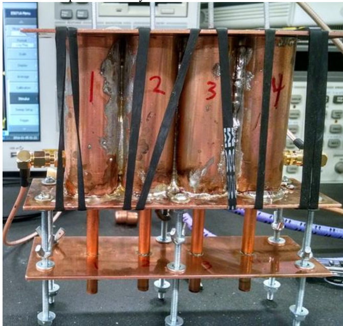
Fig. 12. Final construction of the Cavity Resonator Filter with added tuning screws and adjustable poles
