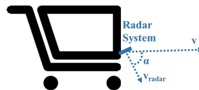
Fig.5 Mounting of Speed Measurement Test
