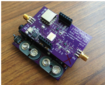
2.4 GHz radar RF and baseband PCB stack-up
