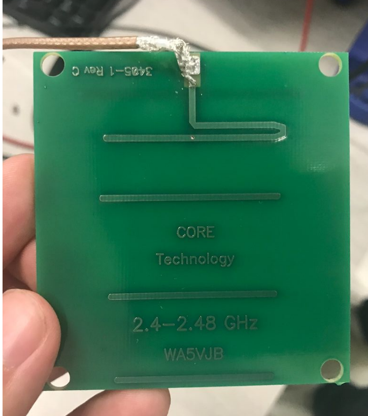
Fig. () Yagi Antenna (Transmit)
