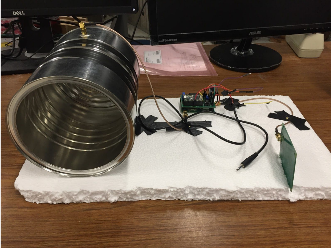
Fig 21: Whole radar system
