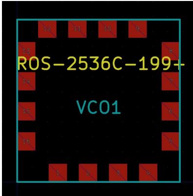
Fig 13: an example of VCO footprint
