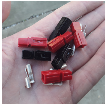
Anderson connectors. Wires solder into the metal lugs, which insert into the plastic sockets. Sockets slide together to make a harness.
