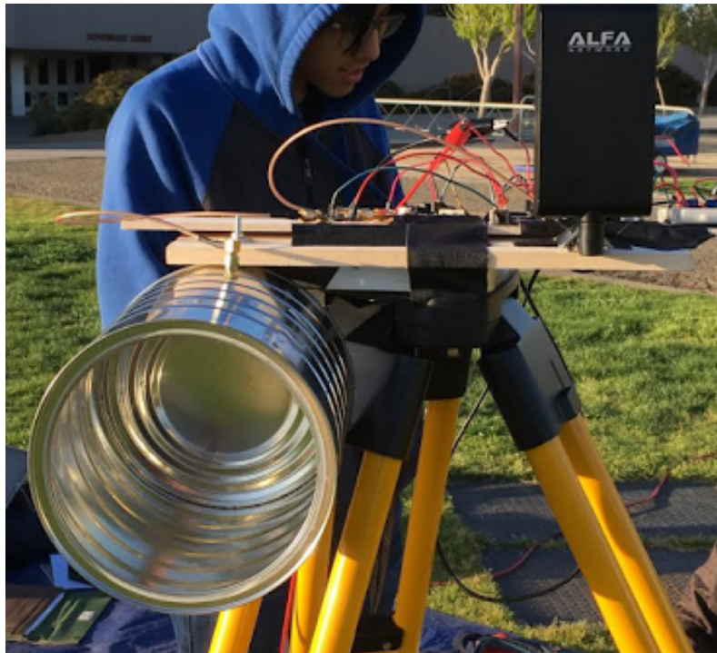
Figure 14. Side view of final implementation with antenna mounts
