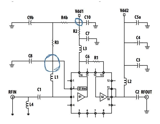
Luckily, the node was related to biasing and not matching. This allowed our group to solder jumper wires in the necessary areas.
