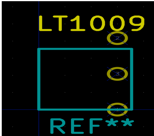
Fig 5. LT1009 Footprint with Error
