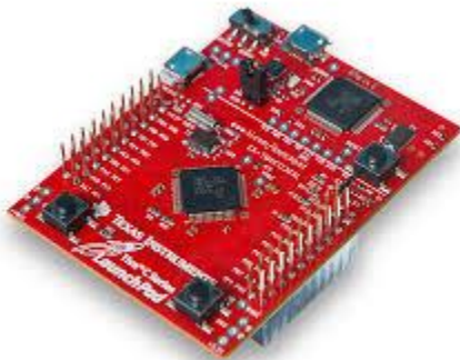
Figure 4: Tiva C Launchpad Microcontroller for DSP
