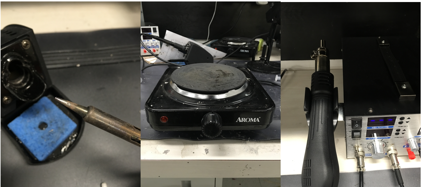
Figure 1. Hot Iron, Hot Plate, Hot Air.
