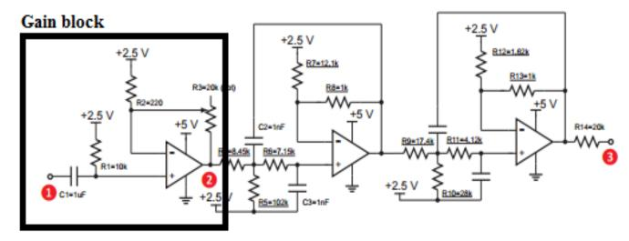
Figure 1: Schematic of Gain stage and LPF
