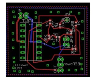
Figure 6: PCB layout for the LPF (34.09 x 30.94 mm)
