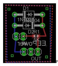
PCB Layout for the voltage limiting circuit (16.10x20.27mm)
