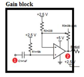
Figure 3: The schematic of the gain stage module
