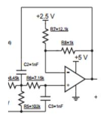
Figure 5: This is the schematic of LPF (two of these schematics with different resistor values)
