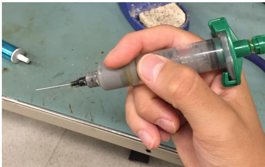
The solder released from the pump is controlled by a foot pedal. The syringe attached to an air pressure line. The foot pedal controls the flow of the solder. Simply press the pedal and this makes the solder paste come out of the syringe at a controlled and steady rate.
