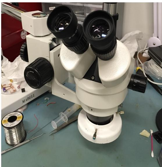
Setting your components on the PCB is a process which involves careful placement of the components onto the pads with solder paste on them. The use of tweezers and a microscope help with the exact placement of your components as shown below.
