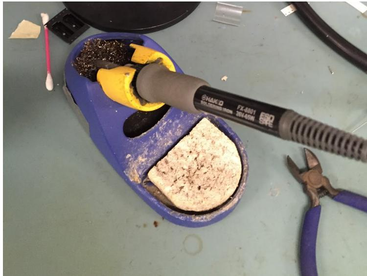
A soldering iron's temperature can be adjusted to allow for different melting points and also to cater towards a device's temperature range in order to avoid damage to the electrical device. In the case of my PCB I adjusted the temperature to around 300 C. The melting point of the alloy tin/lead solder is about 183-188 degrees Celsius.
