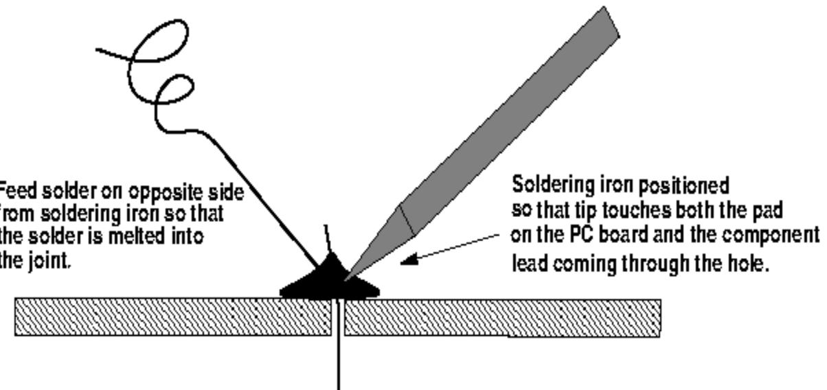
Certain disadvantages of using regular wire solder is that small scale components that needs to be soldered on can't be connected efficiently. The amount of solder applied using wire paste may overflow and may immerse the entire component which can damage most surface mount components. The soldering iron isn't a very precise tool to guide where the solder will be positioned.
