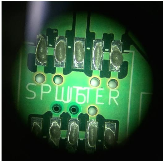
As you can see from the image, there isn't a huge amount of solder paste to saturate the entire pad but there is a healthy amount of solder that when melted will connect the component to the pad.
