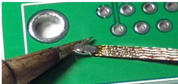
The process of solder wicking is basically defined as solder climbing up on a lead (component, connector, external wire). Wicking is a redistribution of solder away from the intended joint. This is done by placing the wick on the solder which you want to remove. You then place the soldering iron on top of the wick to heat the solder which will be redistributed onto the wick as seen above.
