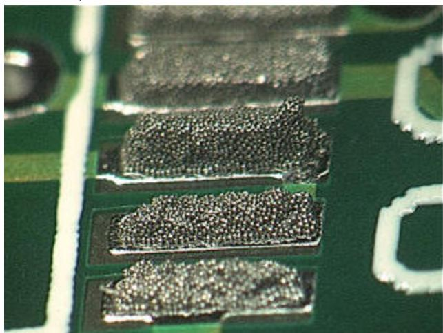
Solder paste contains tiny amounts of solid solder particles mixed together with flux. The advantages of using solder paste can be used to connect smaller scale electrical parts such as surface mount components. Some disadvantages can be that it takes a long time to apply onto the PCB if doing so by hand. If you aren't careful you can misplace the paste and have to reapply after removing the excess amount.
