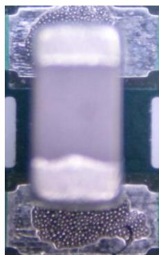
Because each component will be placed one by one with tweezers and the aide of the microscope, you can see how this entire process of soldering surface mounts is extremely time consuming.
