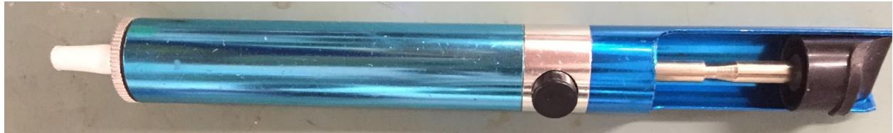
The pump contains a spring-loaded piston which is pushed down and locks into place. When triggered by pressing a button, the piston springs up, creating suction that sucks off the soldered connection. The pump is applied to a heated solder connection, then operated to suck the solder away.
