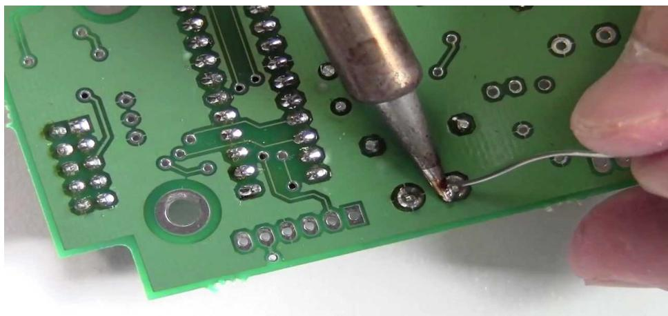
First, you put the leads through the hole. The component needs to be held in place in order for the solder to be applied. You can use clamping devices to hold your PCB down and keep the component from moving.
