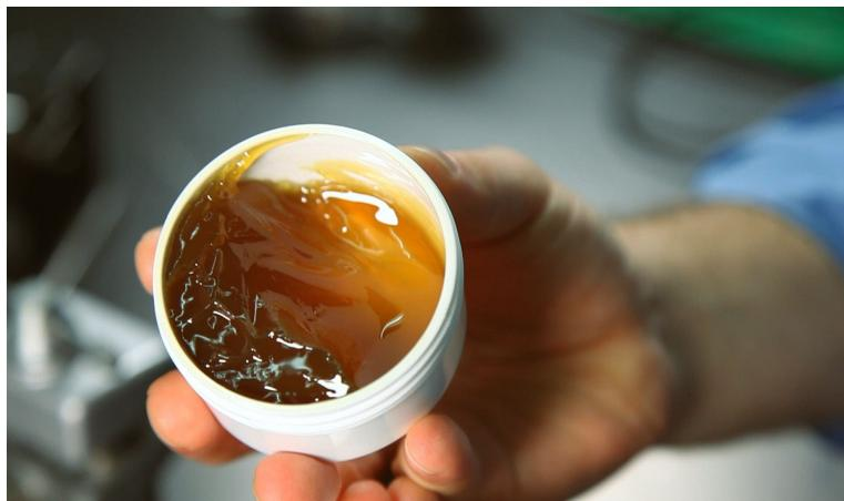
Flux is used as a chemical flowing agent. It reduces the oxides from when the melted solder come in contact with air. The melted solder flows more fluidly when combined with flux. Flux is usually helpful for helping conductivity after applying wire solder. In the case of solder paste, you can apply flux with the solder paste via syringe on the metal contact before you apply the paste.
