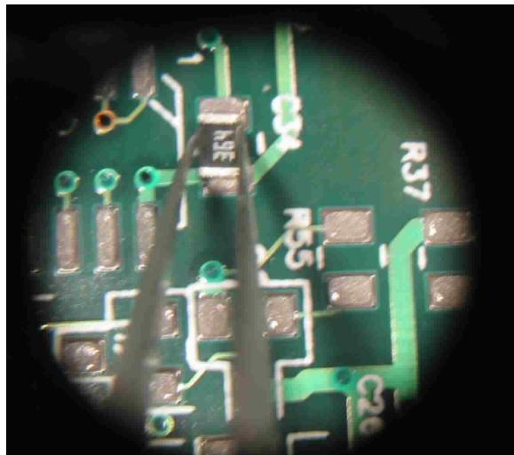
An example of the correct placement of the surface mount component can be seen below when the solder paste is not yet melted.
