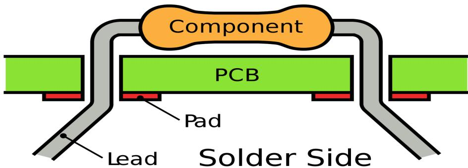
The PCB pads have several holes that the leads of the electrical component can go through. The solder will hold the component onto the board by being applied on the other side where the leads go through the hole. The instrument to apply the solder would be the soldering iron.
